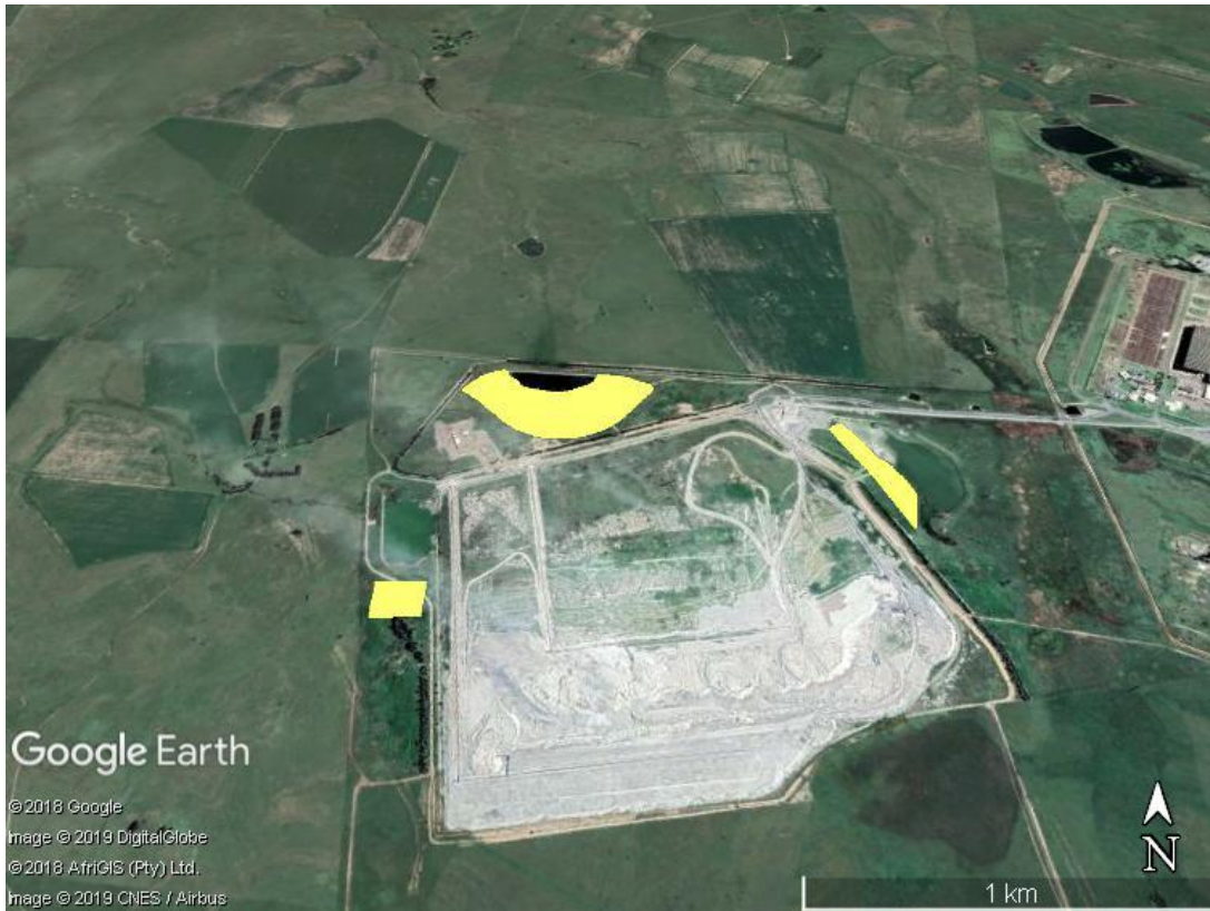
Figure 2: Google Earth Map of the dam sites (yellow) for Majuba Power Station.
