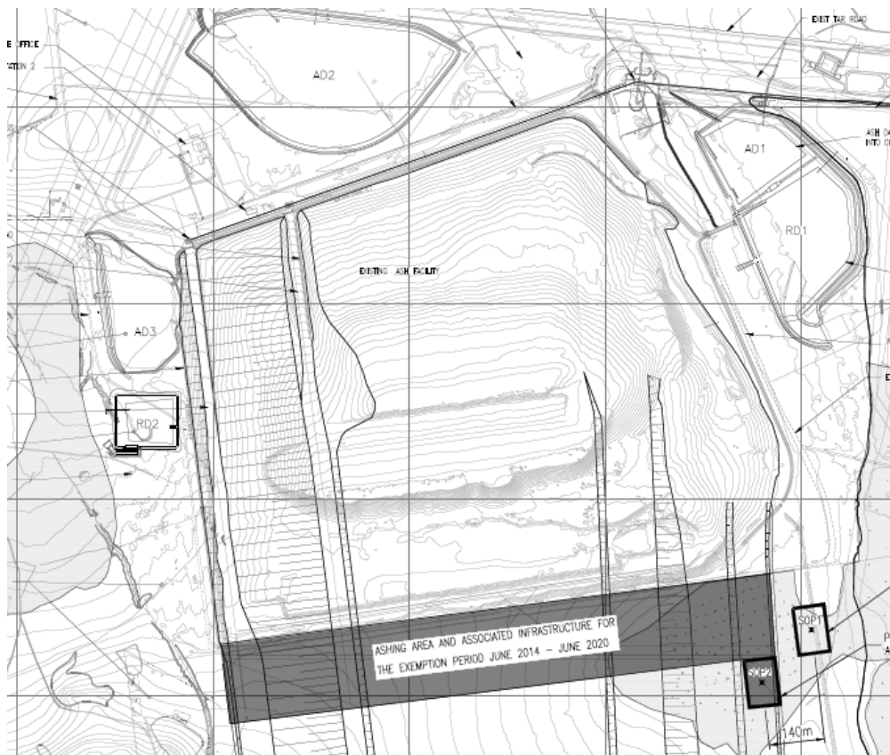
Figure 3: Site plan of four dams, AD3, AD2, AD1, RD1 for Majuba Ash Disposal Facility
